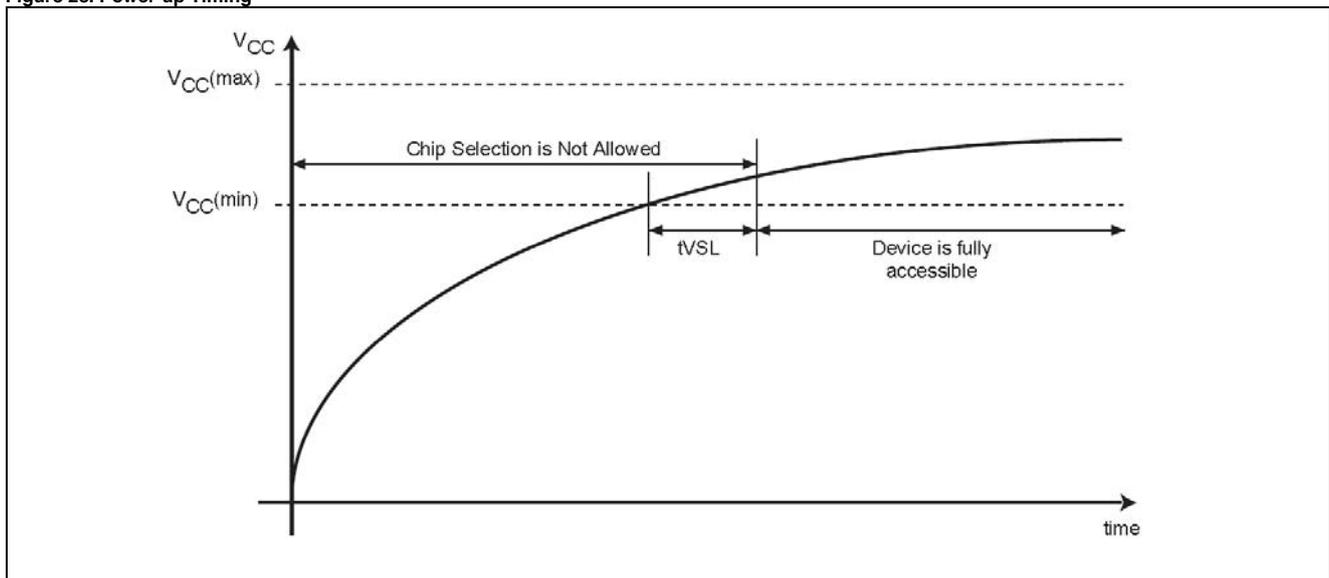
**Note:** VCC (max.) is 3.6V and VCC (min.) is 2.7V.
